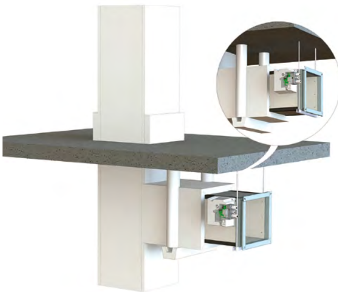
installation of a fire damper
