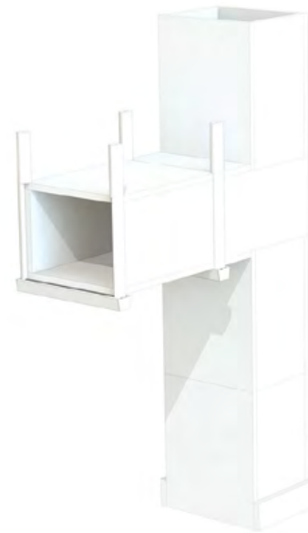
Take-off point on a vertical duct
